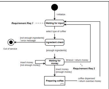
Figure 3 – Example of state transition diagram
