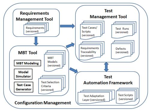
Figure 1 – A typical tool chain embedding MBT
